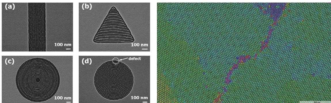
**Left:** Figures a-d, aligned nanowires of platinum, prepared via directed self-assembly. **Right:** large-scale Moiré nanopatterns of  $\sim 10$  nm silica dots with 3-fold symmetry produced through incommensurate block copolymer self-assembly. Scale bar = 500 nm.
