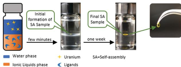
Fig. 1 Self-assembly of the uranium-rich SA sample.
