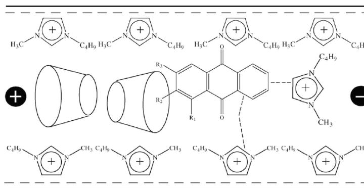
**Fig. (15).** Mechanism of the separation of anthraquinones using C<sub>4</sub>mim<sup>+</sup> based ionic liquid and  $\beta$ -CD. Taken from Ref. [25].
