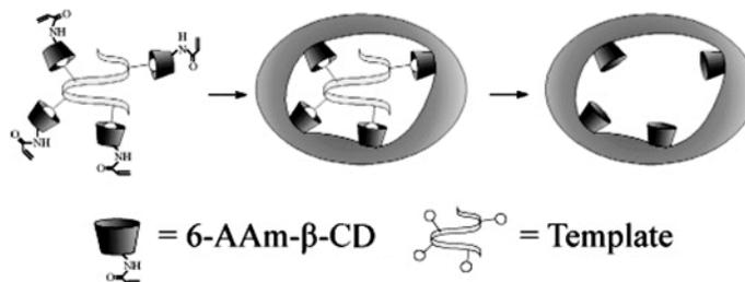
Fig. (8). Schematic view of molecular imprinting of  $\beta$ -CD toward oligopeptide template. Taken from Ref. [57].
