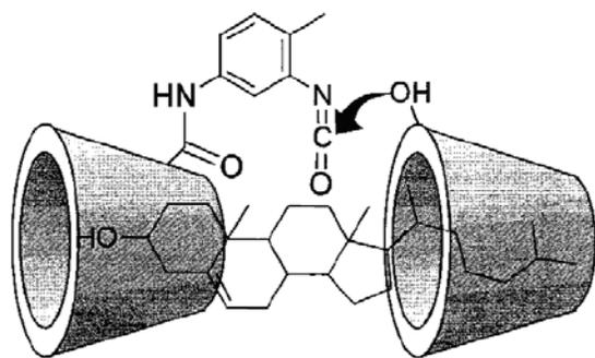
Fig. (3). Proposed mechanism for the molecular imprinting of  $\beta$ -CD with cholesterol (cross-linking agent: TDI). Taken from Ref. [73].
