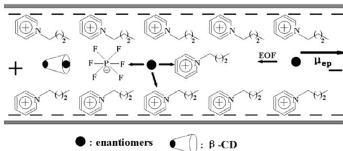
**Fig. (14).** Mechanism of enantioseparation of  $\beta$ -agonists enantiomers using [C<sub>4</sub>Py][PF<sub>6</sub>] with  $\beta$ -CD. Taken from Ref. [100].
