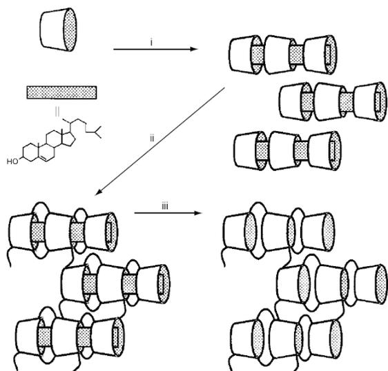
**Fig. (1).** Reagents and conditions of preparing MIP based on  $\beta$ -CD for recognition of cholesterol: i, hexane–H<sub>2</sub>O; ii, diisocyanate in DMSO; iii, acetone, H<sub>2</sub>O, THF, EtOH. Taken from Ref. [55].
