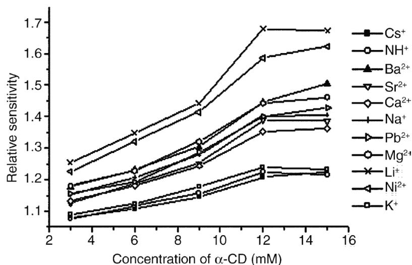
**Fig. (12).** Influence of  $\alpha$ -CD on detection sensitivity of ions; buffer: 7.5mM lactic acid, 0.6mM 18-crown-6, added by desired concentration of  $\alpha$ -CD and adjusted to pH 4.0 by 100mM HMIM hydroxide; capillary: 40 cm; applied voltage: 8 kV; injection: 50 mbar, 15 s; detection: PGD. Taken from Ref. [98].
