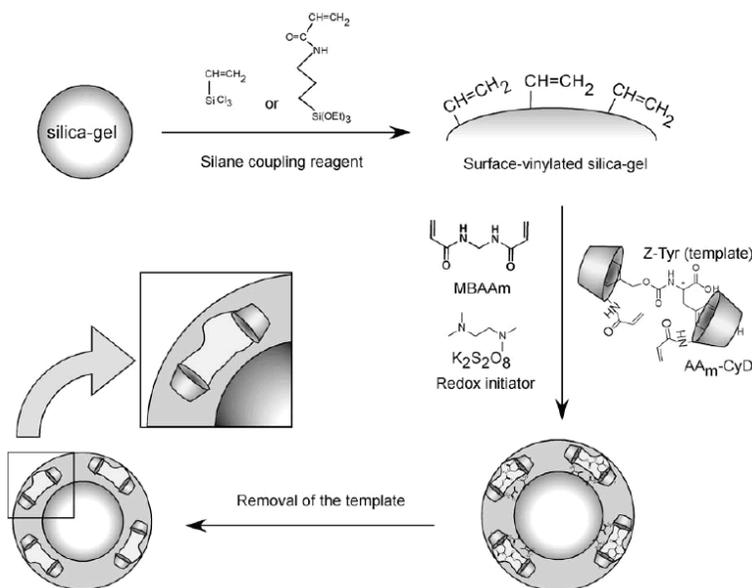
**Fig. (5).** Procedure of the immobilization of imprinted  $\beta$ -CD polymer on silica-gel. Taken from Ref. [85].
