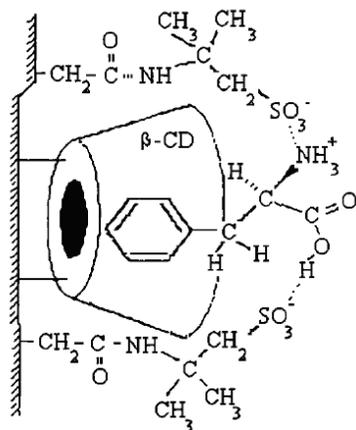
Fig. (4). Schematic illustration of the binding of D-phenylalanine in an imprinted polymer composed of polymerizable  $\beta$ -CD, 2-acryloylamido-2,2'-dimethylpropane sulfonic acid (AMPSA), and *N,N'*-diacryloylpiperazine. Taken from Ref. [74].
