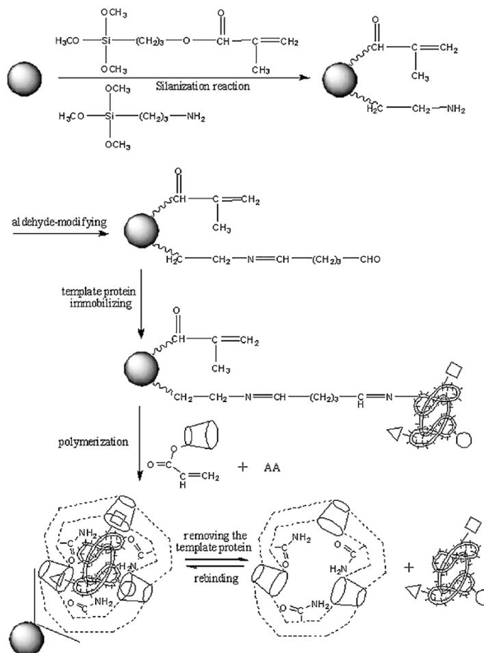
**Fig. (9).** The protocol for synthesis of the protein imprinted polymer. Taken from Ref. [89].
