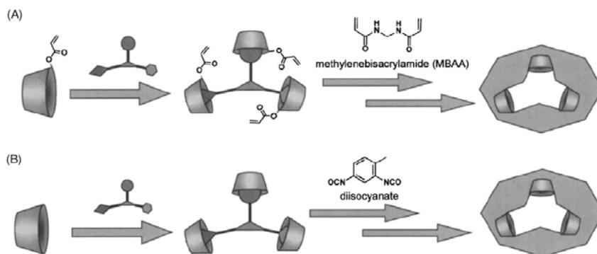
**Fig. (2).** Molecular imprinting of  $\beta$ -CD in water (A) and in DMSO (B). Taken from Ref. [68].
